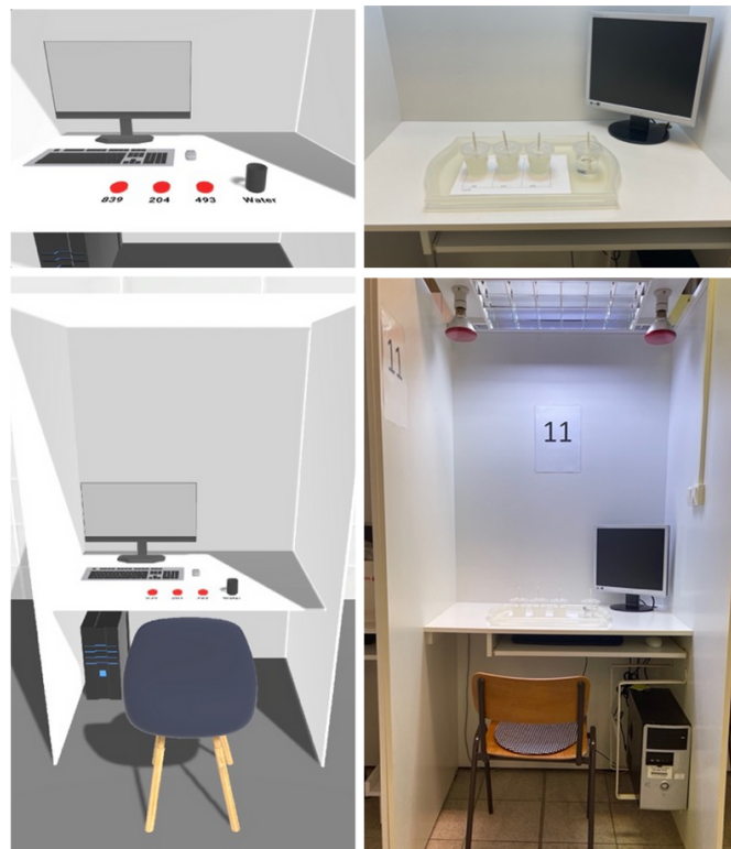
Figure 15: The virtualized sensory lab overview of sensory booth based on ISO standard using Unity.
